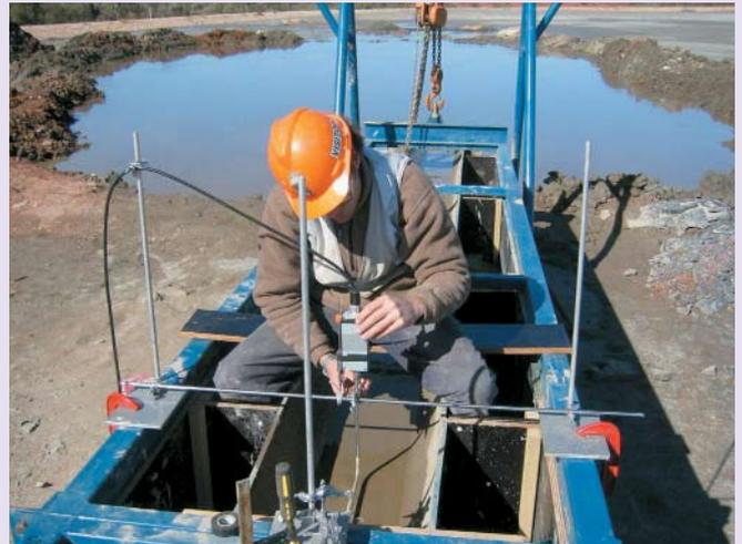
Taking flow velocity measurements in the flume
