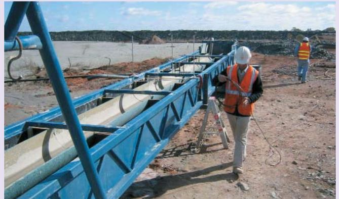
Setting up the flume apparatus at a mine site in Cobar, New South Wales
