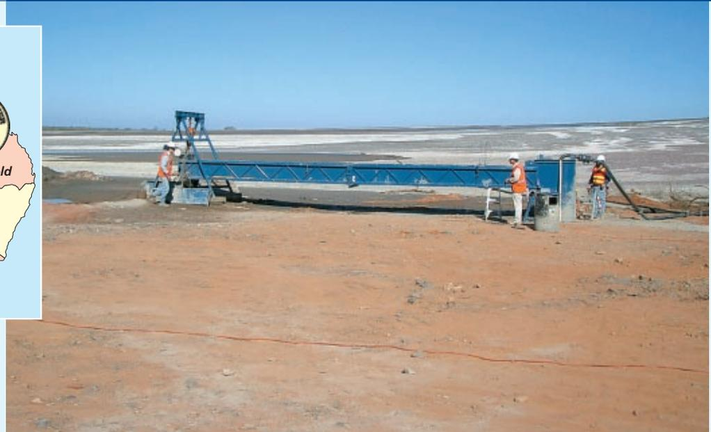
[Right] The beach slope test flume at Peak Gold Mine. The Peak CTD tailings stack is in the background.
