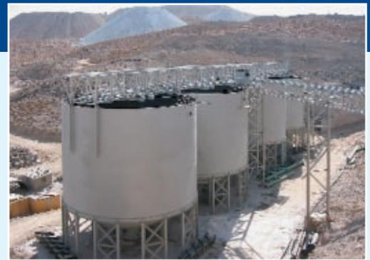
*Deep Cone® Thickeners engineered by GL and V.*
