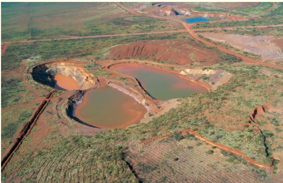
*Newmont's Tanami Operation, Assault [right] and Battery [lower] Pits being backfilled with tailings. Bastille Pit [left] used for stormwater runoff.*
