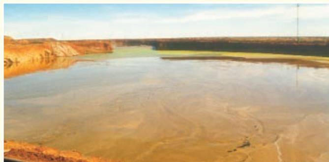
*Bullakitchie Pit at Newmont's "The Granites" Gold Mine during filling. The wet surface is typical of in-pit tailings deposition and is an indication of underconsolidated tailings and considerable future surface settlement.*
