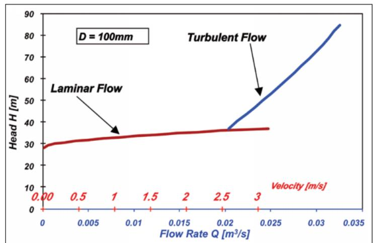
**Figure 2: Pipeline Flow Behaviour of Fine Non-Settling Solids**
