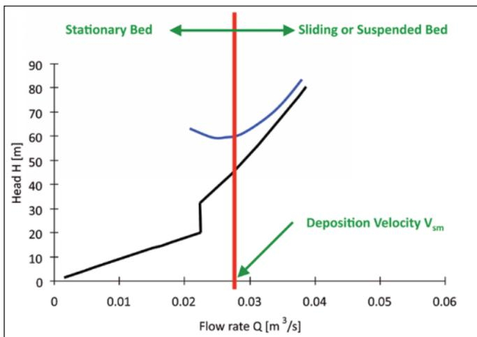
**Figure 1: Pipeline Flow Behaviour of Coarse Settleable Solids**
